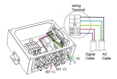
Note: From the state of signal cable, we can know the on and off states of the switch remotely. When the switch is ON, DRY-C1 is connected to DRY-C2; when the switch is OFF, DRY-C1 is disconnected from DRY-C2.
