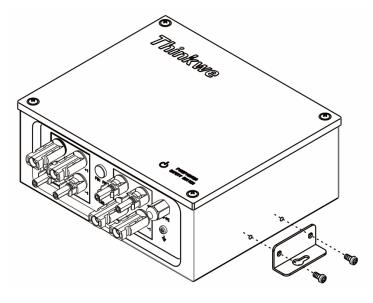
Step 2: Fix the Firefighter Safety Switch on the wall or the solar bracket.
