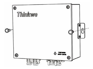
Step 3: Connect the ground cable to the enclosure.
