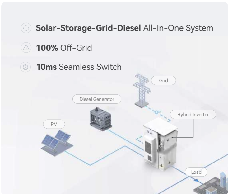
125kW Hybrid Inverter
