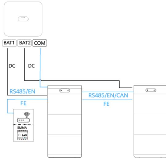
**Figure 2-11** Connecting the ESSs to the inverter (3)
