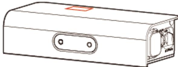
**Figure 2-16** Nameplate position of the Energy Storage Module
