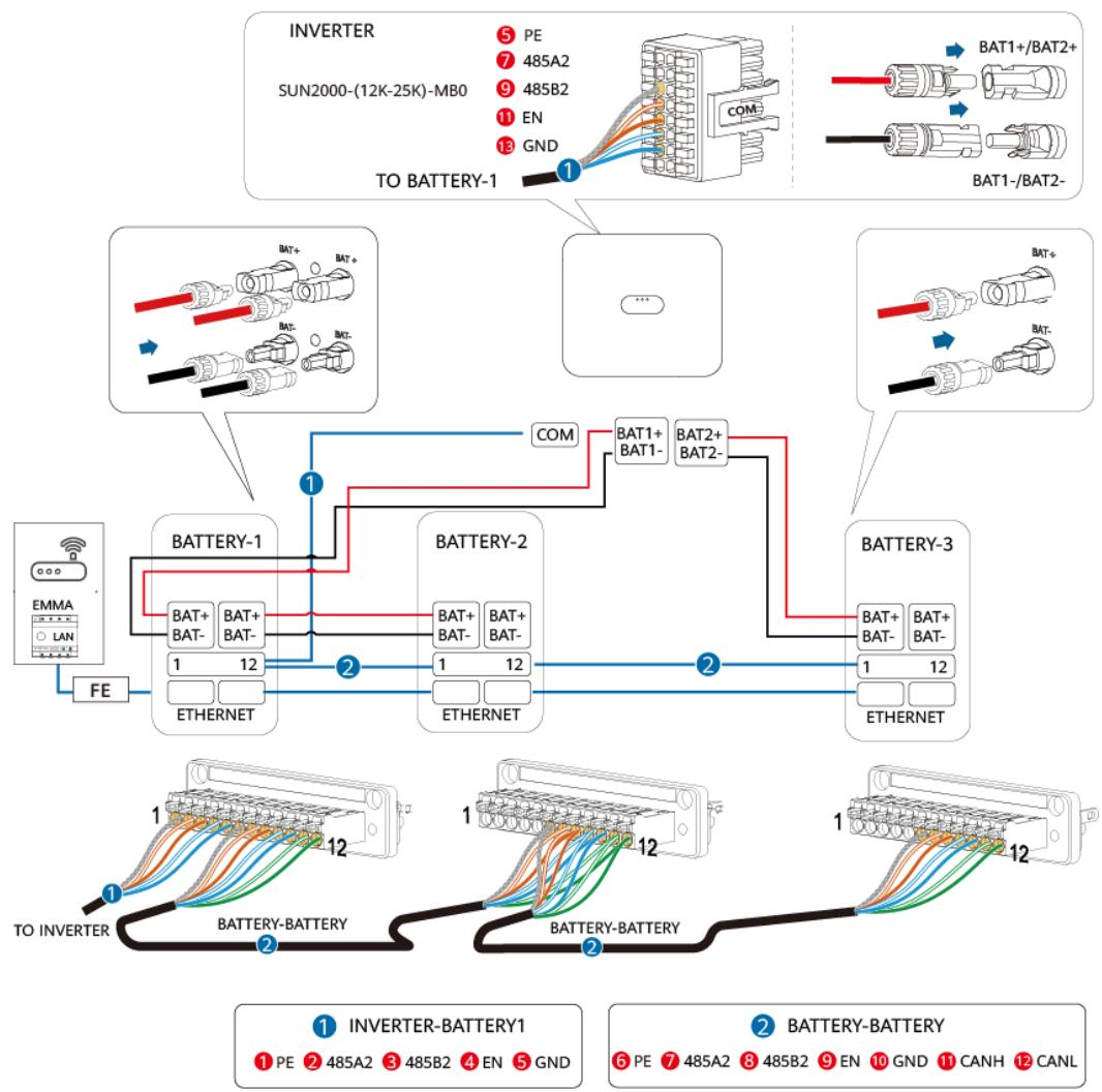
Figure 5-11 Inverter connected to four ESSs
