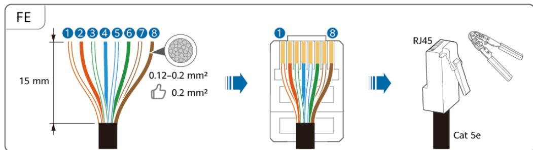
Figure 5-7 Signal port connections
