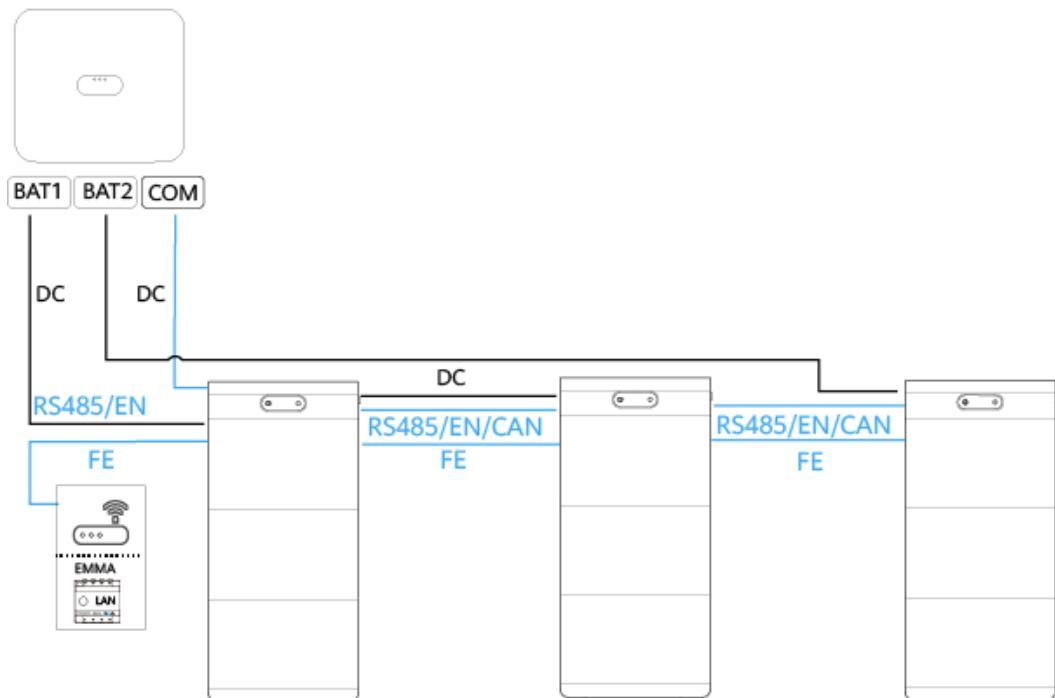
**Figure 2-12** Connecting the ESSs to the inverter (4)
